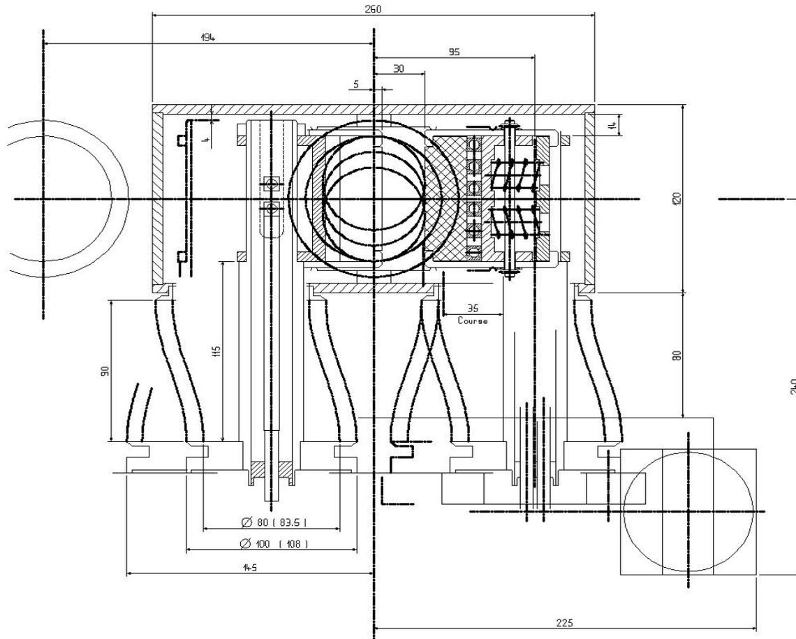
Collimator cross section with spare surface and motorisation. Outer envelope: 450 x 350 mm
