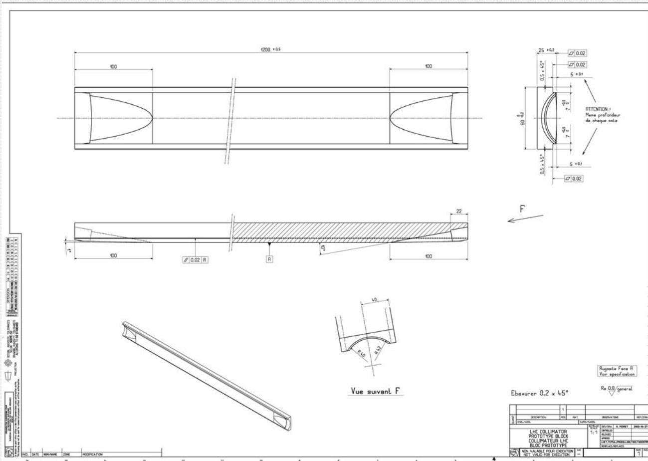
Collimator jaw with tapering
