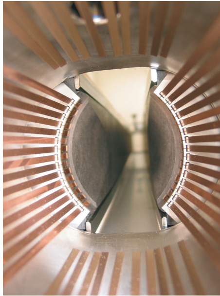
Figure 3.3: RF fingers of a LHC secondary collimator jaw (left and right ones). The set of the external vacuum chamber can also be seen (top and bottom ones). The overall assembly is designed to minimize broad-band impedance and trapped modes due to the movements of the collimator jaw during machine operation [52].
