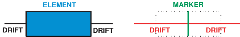
Figure 3.7: Schematic of the thin-lens formalism: the figure on the left reproduces what an element looks like in the lattice, while on the right is shown its thin lens representation. The considered element is replaced by a drift space of equal length, with a marker at the centre stating the name of the element. In that formalism, distances between two consecutive elements are equivalent to the real inter-distance in the lattice plus the respective half-lengths of the two considered elements.
