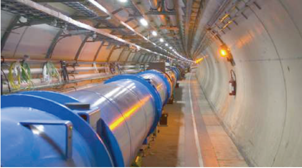
Figure 2.2: Superconducting dipoles in the LHC tunnel.
