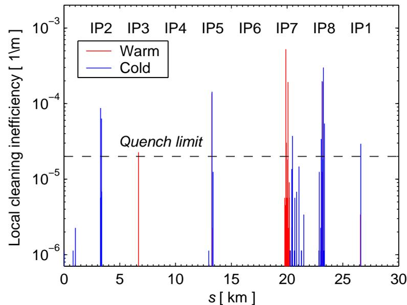
Figure 5: Example of **loss distribution** [5] around the ring for betatron cleaning. The losses are expressed in terms of local cleaning inefficiency and are directly compared to the **estimated quench limit for nominal intensity and a beam lifetime of 0.2 h (design goal)**. Note that all IR's are squeezed to nominal  $\beta^*$ , except IR8 where the initial  $\beta^*$  of 1 m is assumed.
