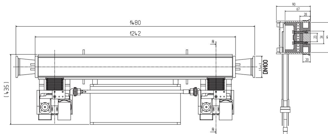
Figure 2 Drawing of the TCS tank (left) and possible Cu/W jaw layout (right) for the TCT collimators at the D2 location [3].
