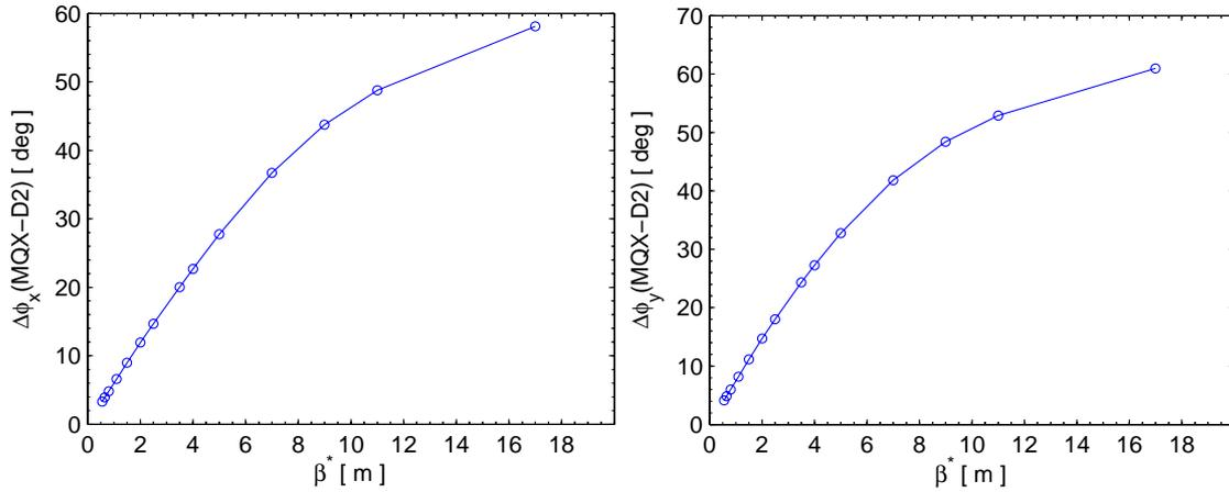
Figure 1 Horizontal (left) and vertical (right) phase advance from D2 to the superconducting triplet, shown as a function of the beta value in the interaction point [2].
