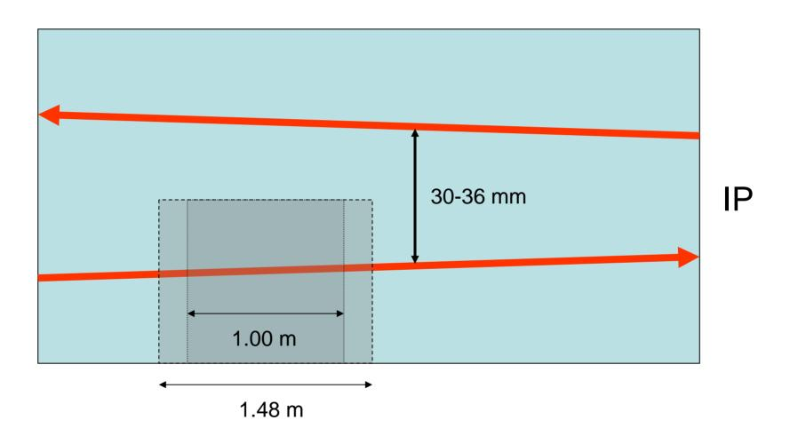
Total length of tank: 1.48 m Length of jaw flat top: 1.00 m
