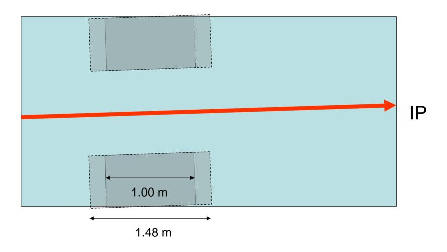
Total length of tank: 1.48 m Length of jaw flat top: 1.00 m
