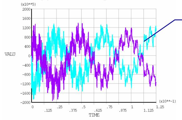
Bending stress at midspan on Cu-strip face
