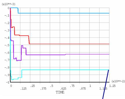
Longitudinal strains are always negative and seem to have stabilized after some millisec.
