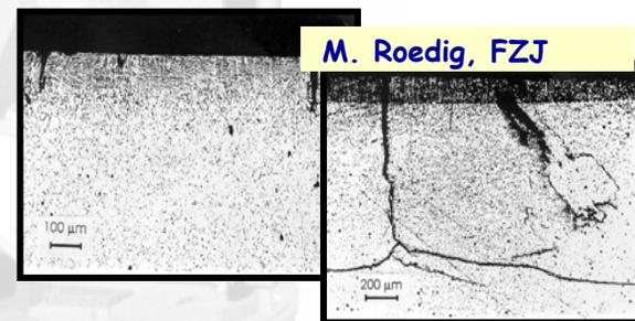
Metallography of S-65C and TR-30 after disruption heat load
