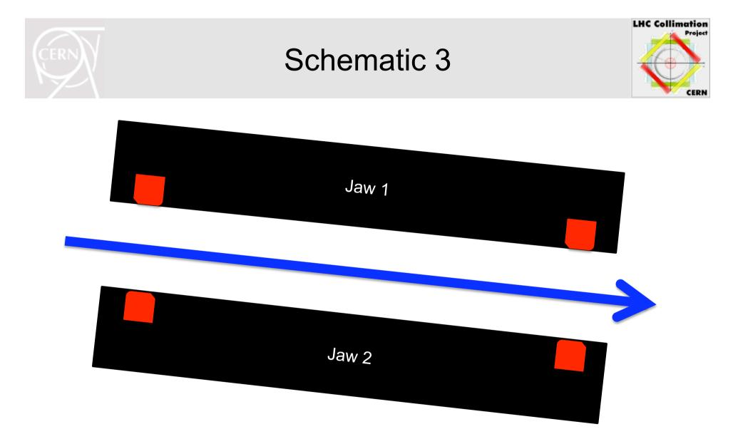
2) Put the same gap at both ends as measured from jaw position (phase 1 feature).
