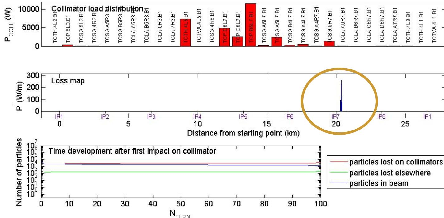
Losses confined to IR7 dispersion suppressor,  $\eta=0.055$
