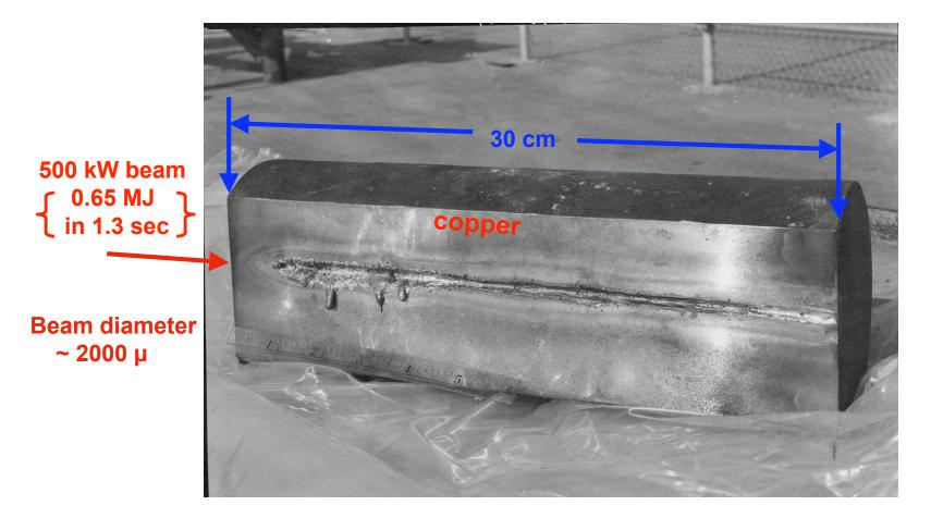
It took about 1.3 sec to melt thru the 30 cm block, but for this relatively large beam, the front two radiation lengths remain intact.
