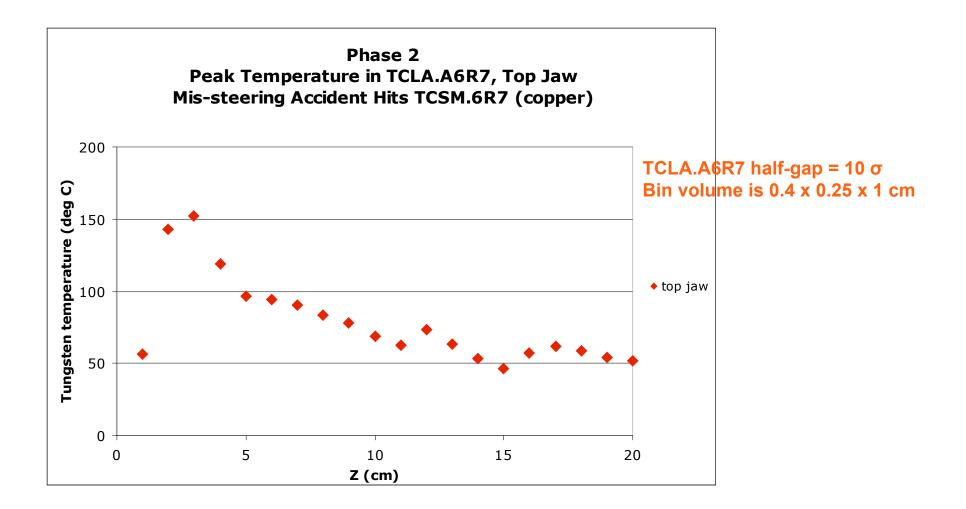
Longitudinal Temperature in TCLA.C6R7 - Accident Hitting TCSM.6R7 - Phase 2
