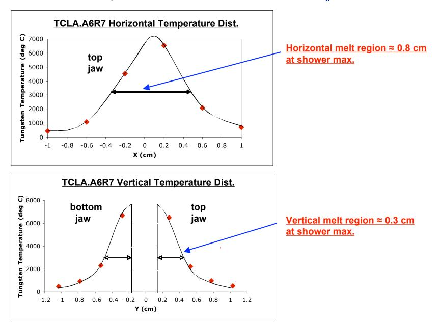
4.2 equivalent bunches hit TCSG.6R7, 7 to 10  $\sigma_x$
