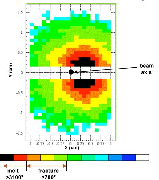
4.2 equivalent bunches hit TCSG.6R7, 7 to 10  $\sigma_{x}$
