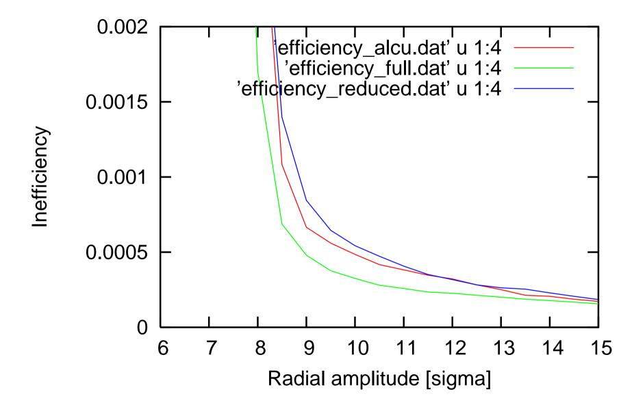
Efficiency at 10 sigma (7 TeV) roughly the same as with the Al/Cu system! Larger impact parameters (results in larger tolerances).
