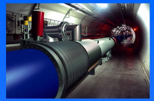
Illustration of LHC dipole in tunnel
