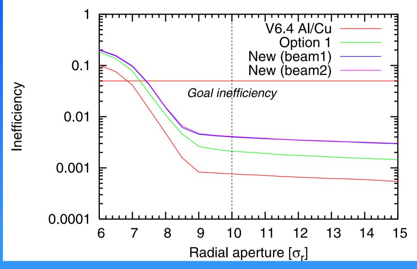
Loose factor 4 in inefficiency (factor 2 with respect to feasible solution) but stay factor 10 below goal inefficiency!
