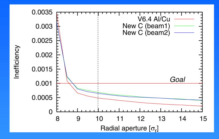
Inefficiency at  $10\sigma$  about 40% higher than in old solution, but well below the target inefficiency! Beam1 and beam2 solutions show same efficiency!
