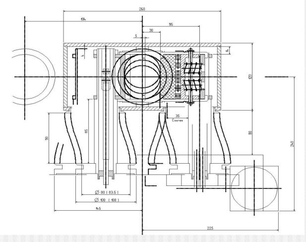
Collimator cross section with spare surface and motorisation. Outer envelope: 450 x 350 mm
