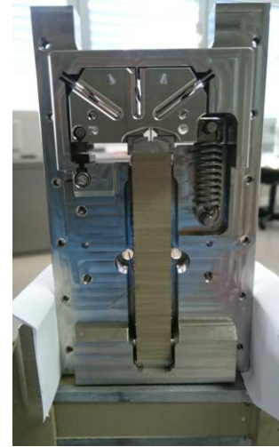
High stiffness rotational stage (V2) used in Beam 2 goniometers.
